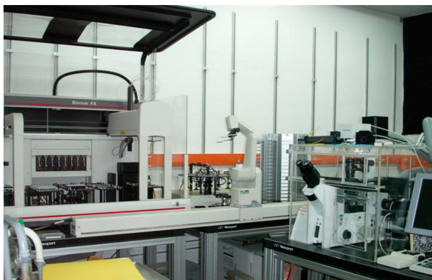
Fig. 2 A photograph of our laboratory, showing the liquid handling robot for culturing cells in multi-well plates, and one of the automated screening microscopes.
