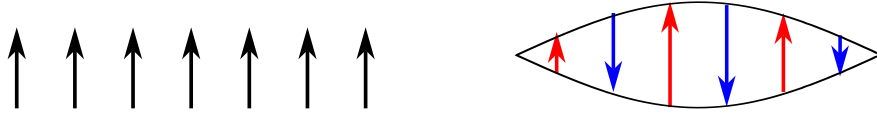
FIG. 1 Schematics of the spatial profile of the most superradiant (left) and most subradiant modes (right).
