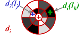
Figure 7. Computing attraction repulsion matrix W : The log-polar self-similarity descriptor d_i is located at l_i (red cross). White bins signify image areas of high similarity to the central patch, dark bins signify image areas of dissimilarity to the central patch. The point l_j (blue cross), which is the center of descriptor d_j (not drawn), falls in a white bin of descriptor d_i (i.e., 0 < d_i(l_j) \leq 1 ). The entry w_{ij} in the matrix W is determined accordingly: w_{ij} = \alpha_{ij} (d_i(l_j) + d_j(l_i)) / 2 , where \alpha_{ij} (the certainty assigned to this entry), is inversely proportional to the distance \|l_i - l_j\| (the distance between the red and blue crosses). Similarly, the point l_k (green cross), which is the center of another descriptor d_k (also not drawn), falls in a dark bin of descriptor d_i , i.e., -1 \leq d_i(l_k) < 0 , and \alpha_{ik} < \alpha_{ij} (because the green cross falls farther away from the center of d_i , hence lower certainty).
