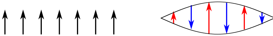
Figure 7.3: Schematics of the spatial profile of the most superradiant (left) and most subradiant modes (right).
