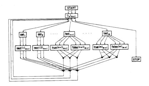
where  $p_1, p_2 ...$  are new variables and F is an arbitrary flowchart. An interpretation is called *nice* if the  $p_i$  range over the domain {true, false} and the test  $p_i$ ? is true (i.e., evaluates to 1) iff the value of  $p_i$  is true. Denote the set of nice interpretations by NICE. Then the Boolean version of our Folk Theorem states:
