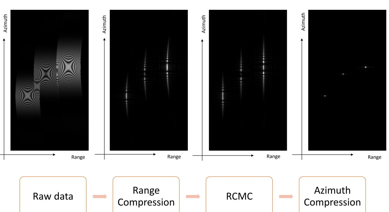
The **RCMC** stage is aimed at decoupling the dependency between the azimuth and range axes and to correct the hyperbolic trajectory of the targets' echoes. The non-constant, non-integer shifts at the RCMC stage are realized by a digital subsequent interpolation which effectively increases the sampling rate of the system.
