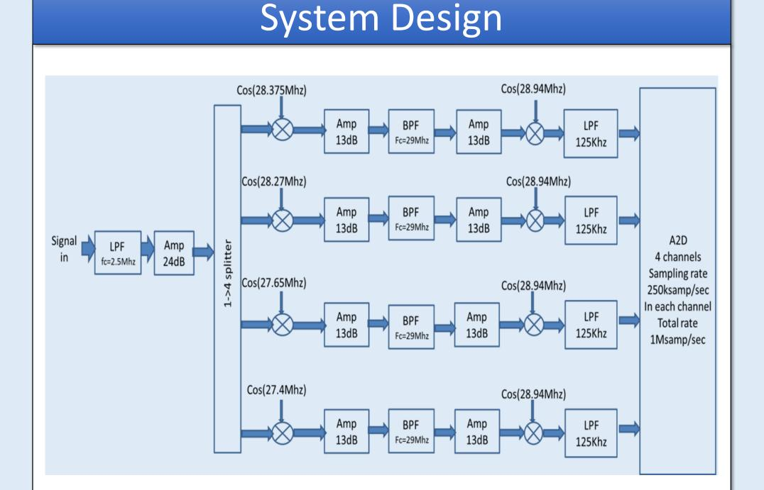
Multi-channel design for 4 transmit subbands
