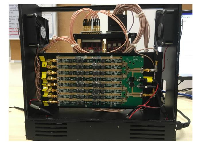
Separate filtering of I and Q signals
