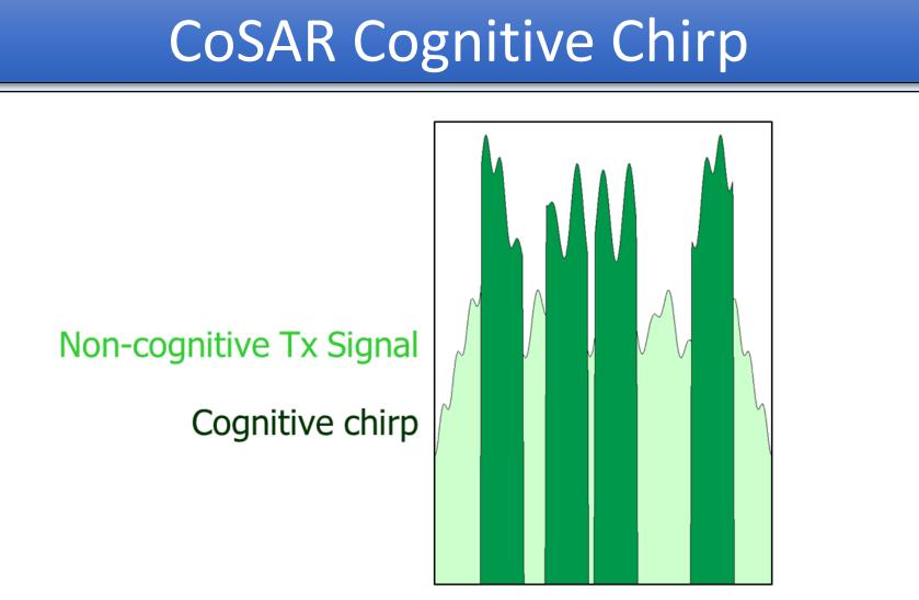
Cognitive chirp signal is obtained by filtering a few subbands of the stripmap SAR Tx signal
