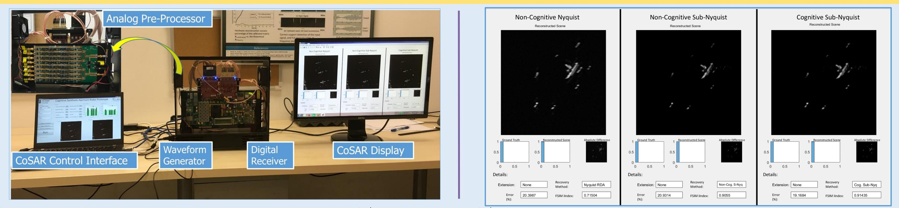
CoSAR recovers the target scene sampled at 1/4<sup>th</sup> and processed at 1/8<sup>th</sup> of the Nyquist rate with least error and most similar low-level features
