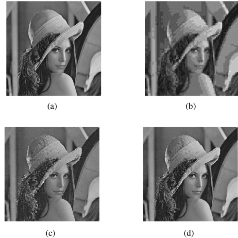
Fig. 8. Image compression. (a) The original image; (b) The compressed image via DCT; (c) The compressed image via joint sampling and quantization with identical quantizers; (d) The compressed image via Algorithm 1.
