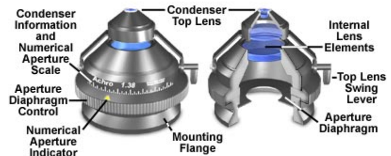
Swing-Out Top Lens Condenser (Numerical Aperture = 1.35)
